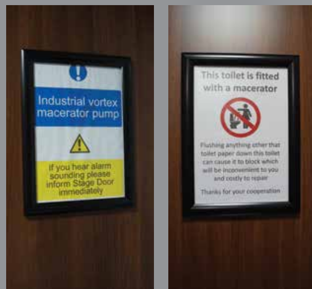
Clear information is now given to the users about items that can be disposed of via a macerator and the chance of an audible alarm warning in the event of a malfunction. The Sanicubic 2 XL can in fact deal with larger items, but the maintenance team is now trying to eliminate the flushing of items other than tissue and waste.
